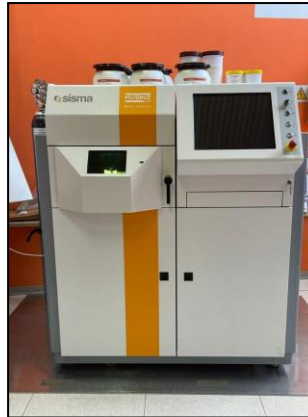
Fig. 1 MYSINT100, 3D selective laser melting printer for metal powder employed for the fabrication of Cu/CNTs nanocomposites.
