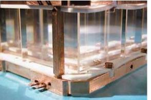
Detail of the dioxide tellurium crystals of the experiment CUORE for the search of double beta decay without neutrinos.
