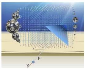
The underwater detectors of the K3 experiments reveal cosmic neutrinos through the Cerenkov radiation emitted by muons during the interactions.
