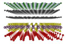
Scheme of a superstructure built from different two-dimensional crystals: going from bottom to top a layer of black phosphorus, of molybdenum disulphide, two layers of graphene and finally a layer of nitride of hexagonal boron are stacked.
